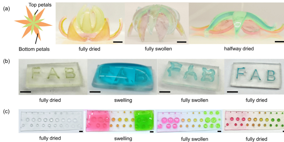
Fig. 5. Illustration of bilayer 3D shape changing objects. (a) Blooming flower 2D pattern and 3D object when fully dried, fully swollen and half-way dried. (b)–(c) PAAm hydrogel letters and pillars bonded on PDMS substrates, and the surface texturing and wrinkling induced by humidity. The scale bars represent 4 mm.
